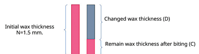
Figure 2: The calculation of the wax thickness change ( D ).
