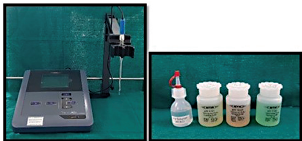
Figure 3: pH meter with microelectrode.
